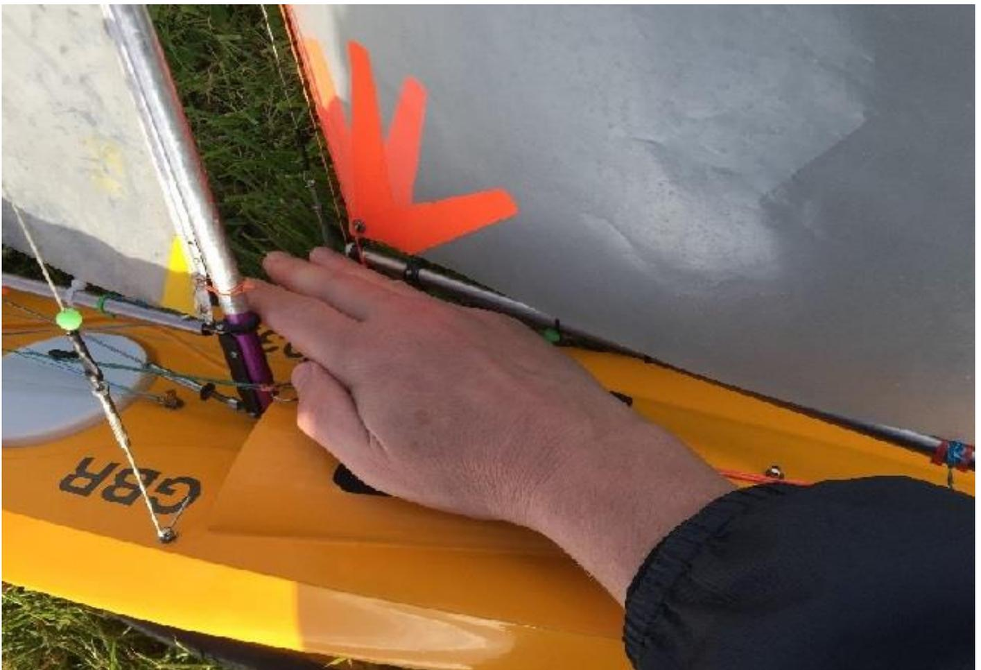
Initial '3 – Finger Rule' when setting the jib slot.
