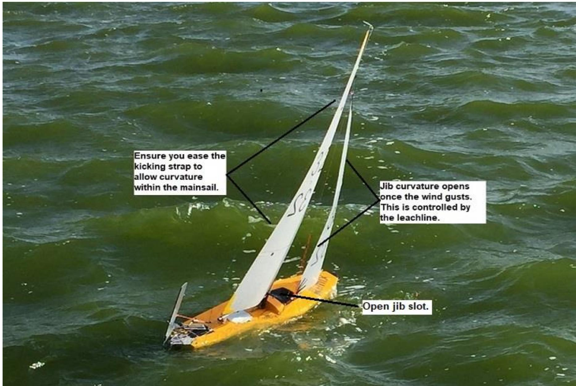
Ensure you ease the kicking strap to allow curvature within the mainsail.
