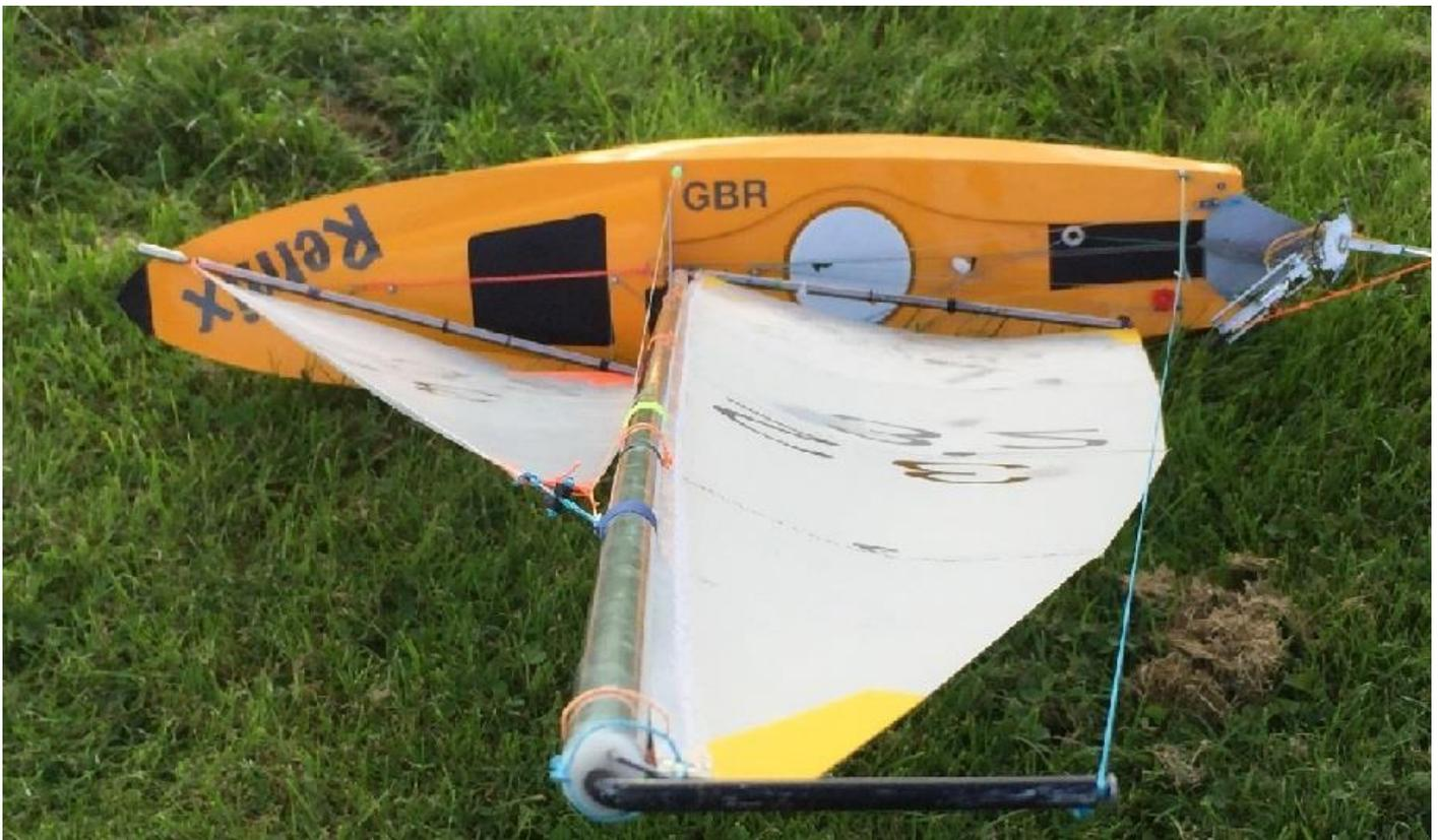
Aim to have a straight mast with some back bend observed in the top third of the rig.
