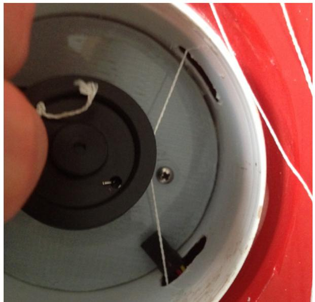
Place the drum on the spindle.
